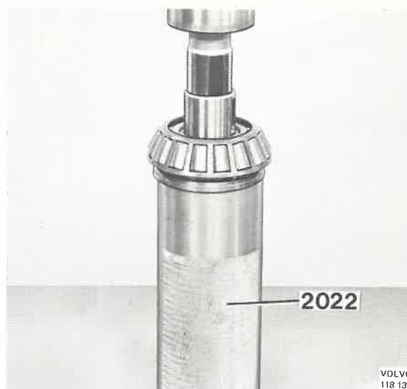
Fig. 92-67. Pressing off the bearing (input shaft)
