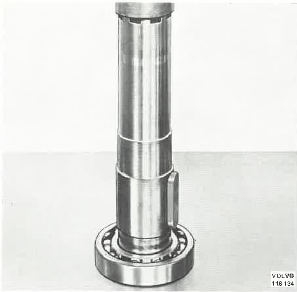
Fig. 92-70. Pressing on the bearing
