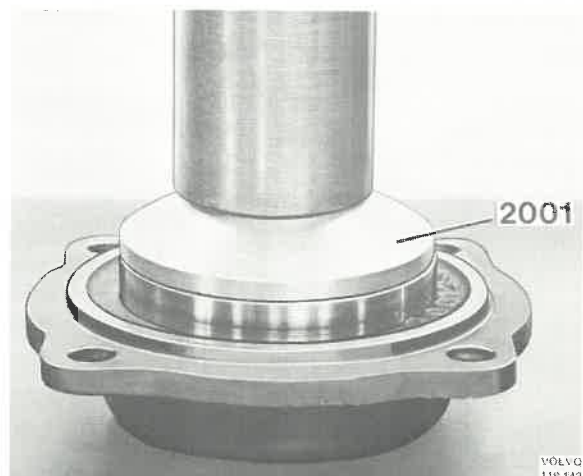
Fig. 92-79. Pressing in the outer race
