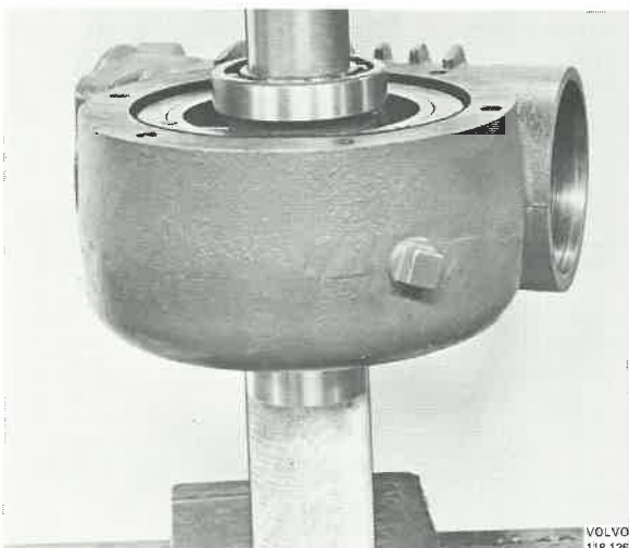
Fig. 92-72. Pressing in the worm gear
