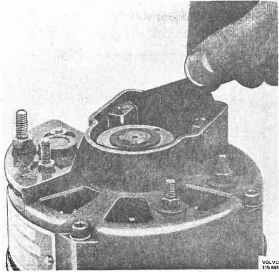
Fig. 32-10. Removing the insulation plate
