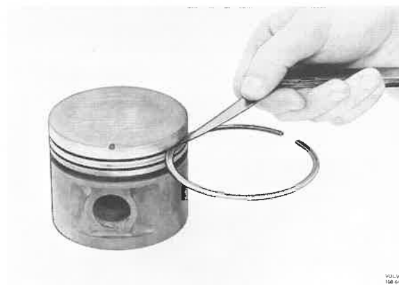
Fig. 21–28. Measuring the piston ring clearance in groove
