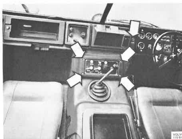
Fig. 26-7. Removing the cover over the radiator and the panel for the diff. lock controls
