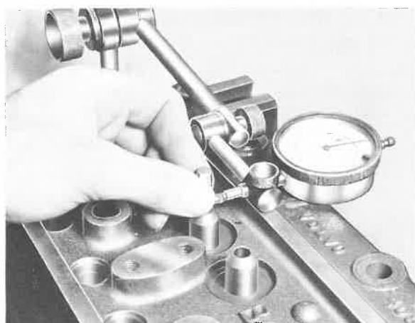
Fig. 21–21. Measuring the clearance between guide and valve stem
