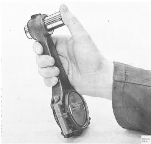
Fig. 21-30. Gudgeon pin fit
