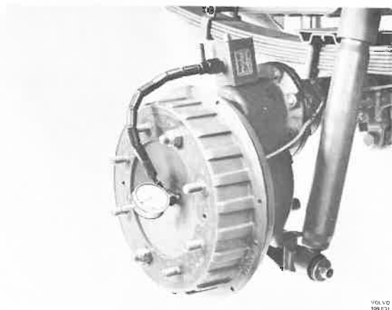
Fig. 77-4. Checking wheel bearing clearance
