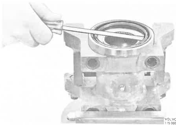
Fig. 76-7. Removing the sealing ring
