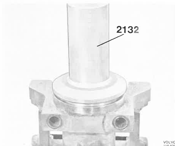
Fig. 76-11. Installing the sealing ring
