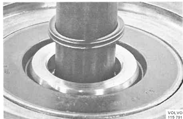
Fig. 46-118. Installing the X-ring
