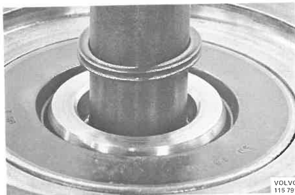
Fig. 46-129. Installing the X-ring
