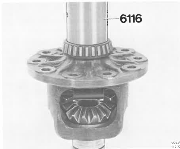
Fig. 46-55. Pressing on the bearing
