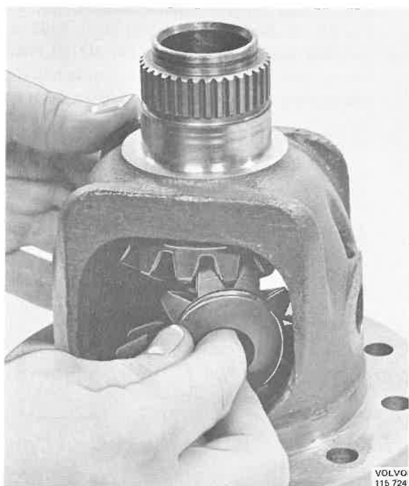
Fig. 46-52. Fitting the diff. side gears
