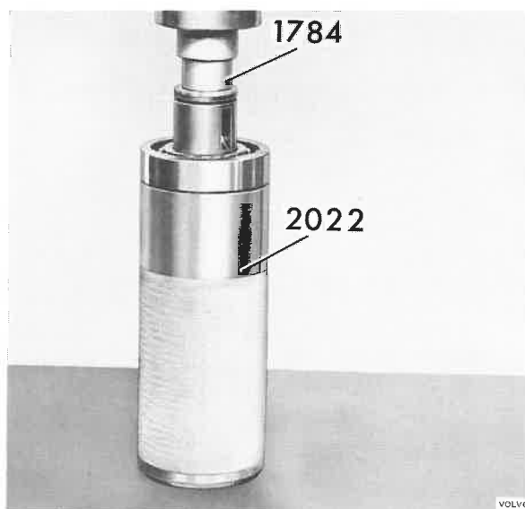
Fig. 48-19. Removing the bearing
