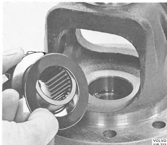
Fig. 46-51. Fitting the thrust washers
