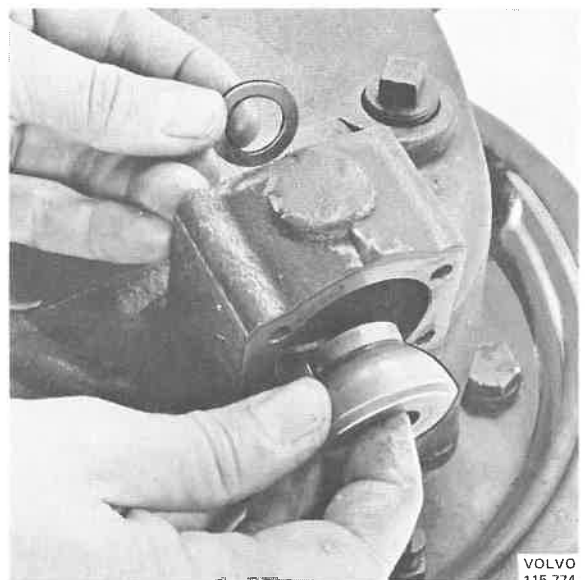
Fig. 46-106. Installing the ball shell
