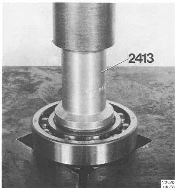
Fig. 46-123. Removing the bearing
