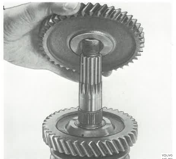
Fig. 43-87. Installing reverse gear
