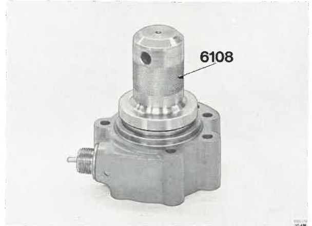
Fig. 43-205. Driving in seal
