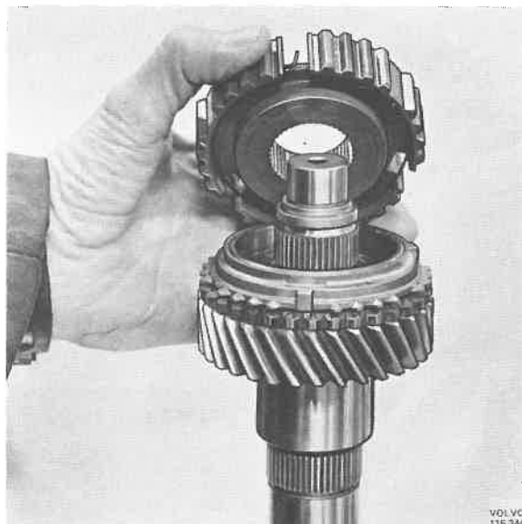
Fig. 43-81. Installing synchronizing hub
