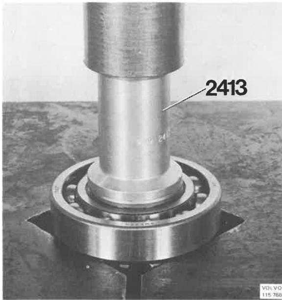
Fig. 46-99. Removing the bearing
