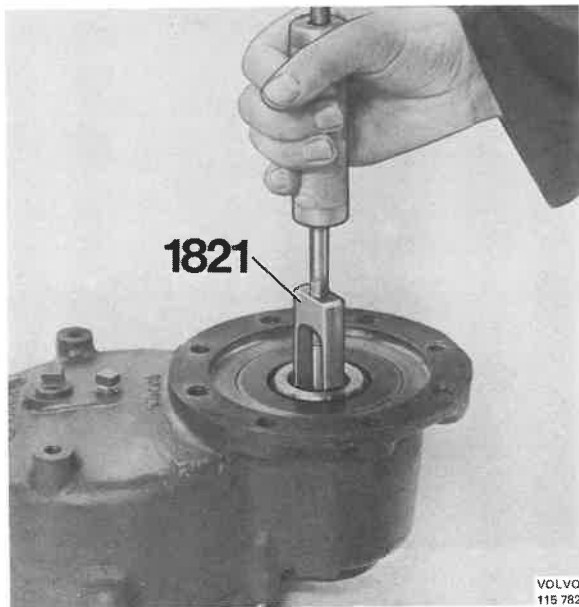
Fig. 46-119. Removing the wear ring
