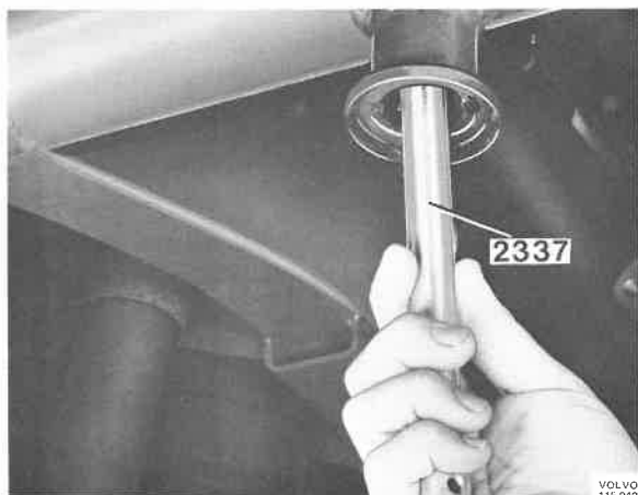
Fig. 64-27. Removing the upper bushing
