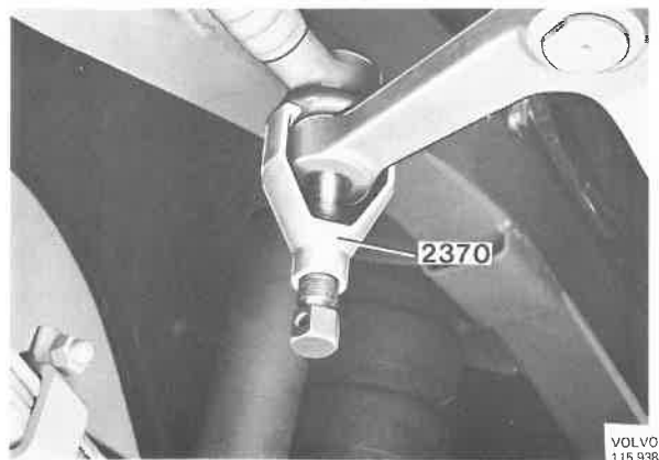
Fig. 64–25. Removing the steering rod
