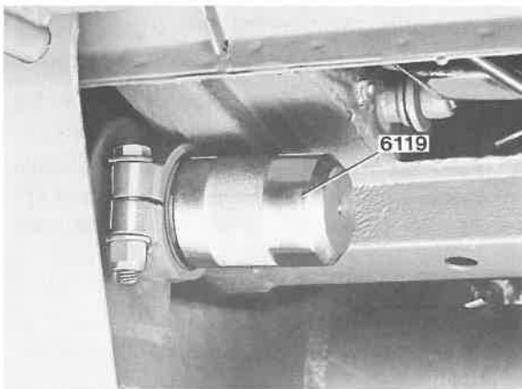
Fig. 64-6. Fitting the sealing ring
