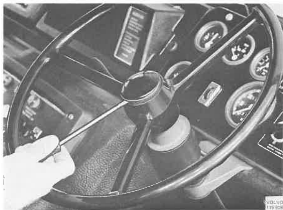
Fig. 64-8. Removing the horn button
