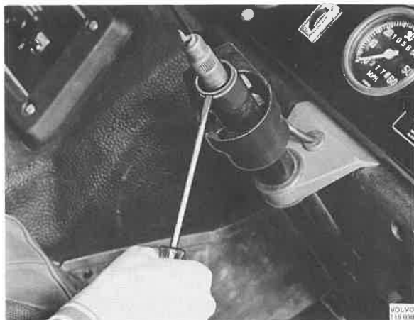
Fig. 64-10. Removing the upper steering shaft bearing
