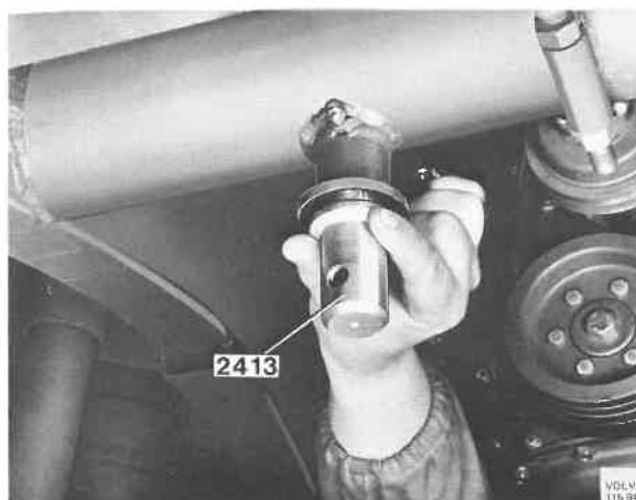
Fig. 64-29. Fitting the bushings
