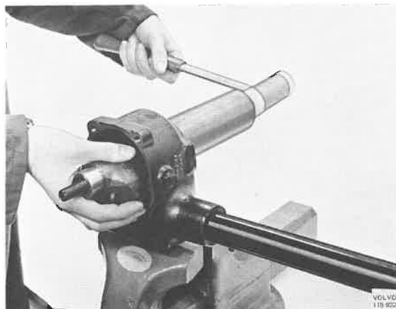
Fig. 64-13. Removing the sector shaft
