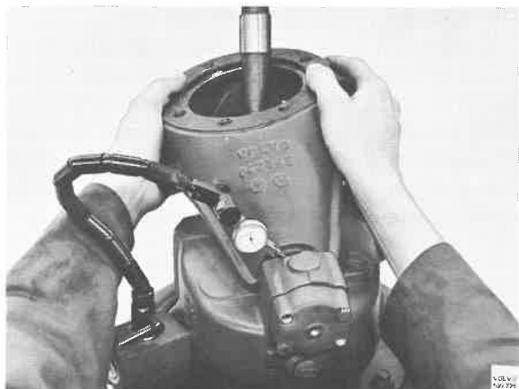
Fig. 63-13. Measuring the axial clearance
