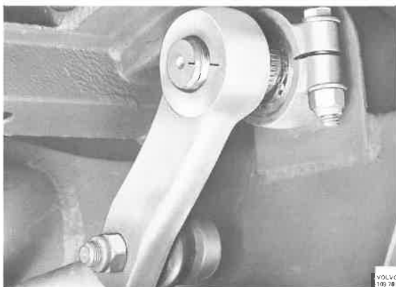
Fig. 64–24. Marking up pitman arm – sector shaft
