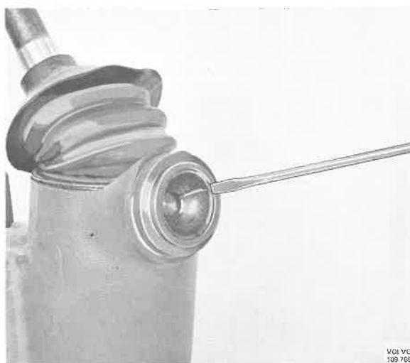
Fig. 63-6. Removing the upper bushing
