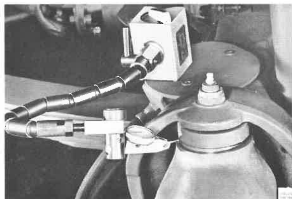
Fig. 63-2. Placing the dial indicator
