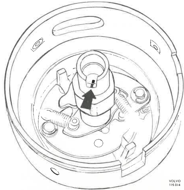
Fig. 34-11. Marking breaker cam and distributor shaft
