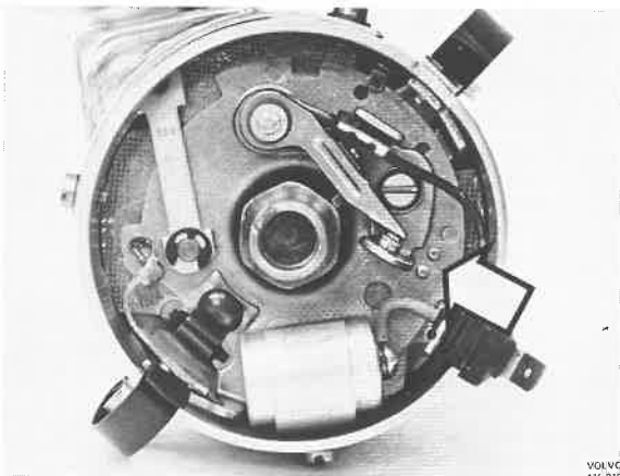
Fig. 34-16. Recess for dwell angle
