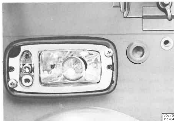
Fig. 35-5. Side and direction indicator bulbs
