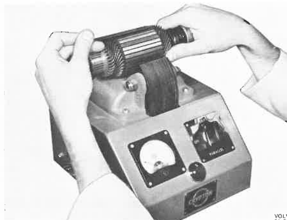
Fig. 33-18. Testing the rotor
